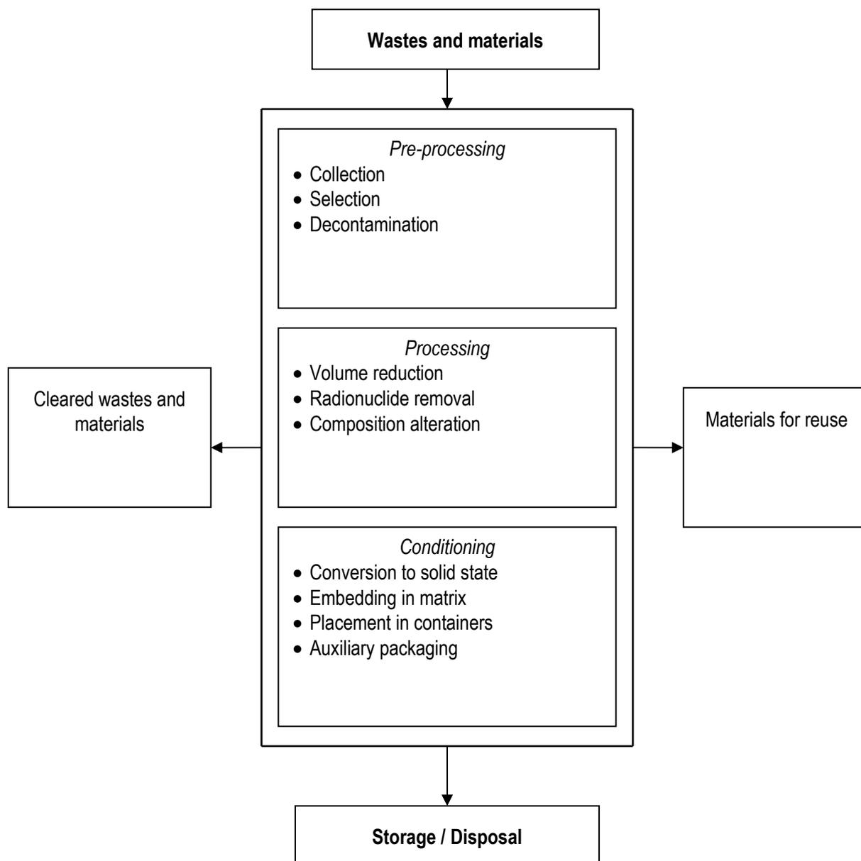
Figure 19.3.5-1: The main phases of radioactive waste management. [19-22]
