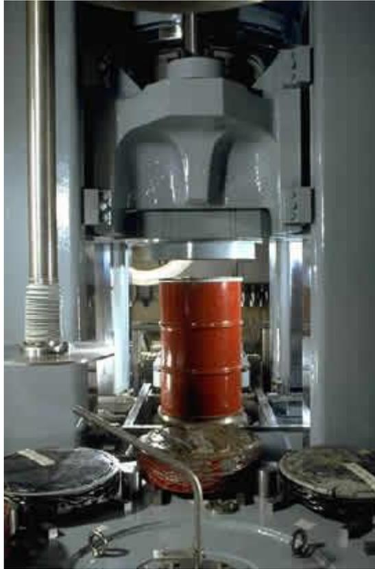
Figure 19.3.5-6: Supercompaction machine and pellet storing unit. [19-6]
