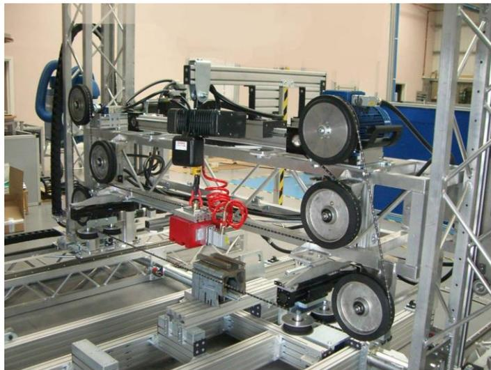
Figure 19.3.5-4.: Diamond rope cutting apparatus. [19-4]
