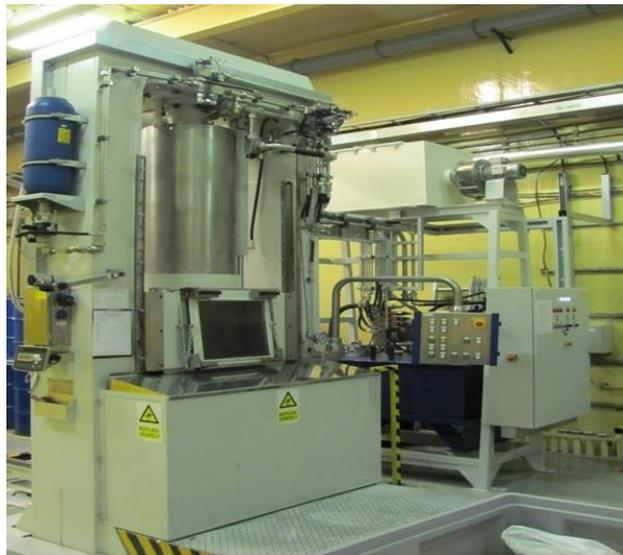
Figure 19.3.5-5: 50 kN automatic waste compaction press. [19-5]
