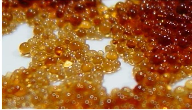
*Figure 19.3.5-10: Inorganic ion exchange resin. [19-10]*
