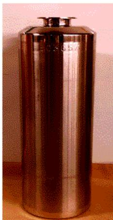
Figure 19.3.5-14: Container holding vitrified waste. [19-32]
