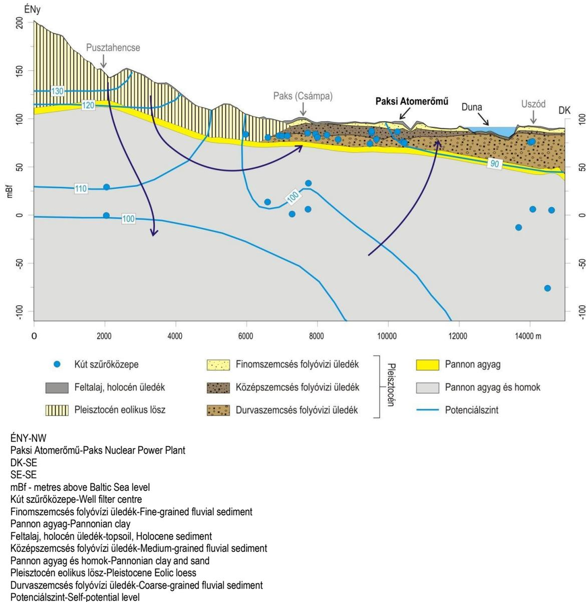
Figure 14.2.2-2: Self-potential log crossing the Paks Nuclear Power Plant
