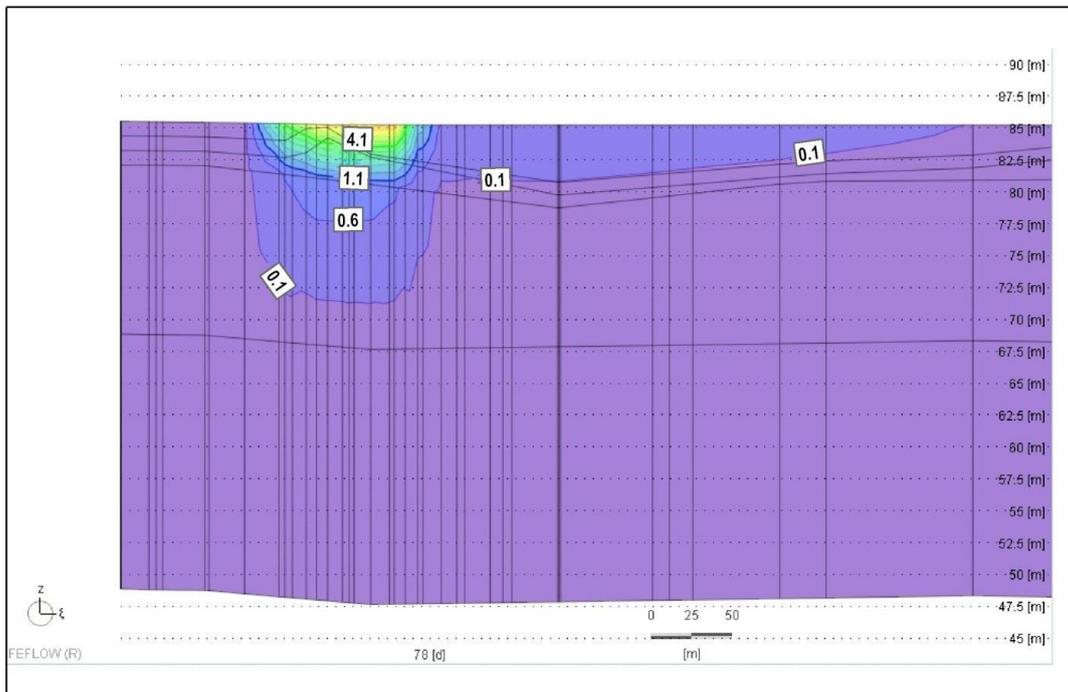
Figure 14.4-9: Modelled temperature change in the Danube and the underground water in the section of warm water influx
