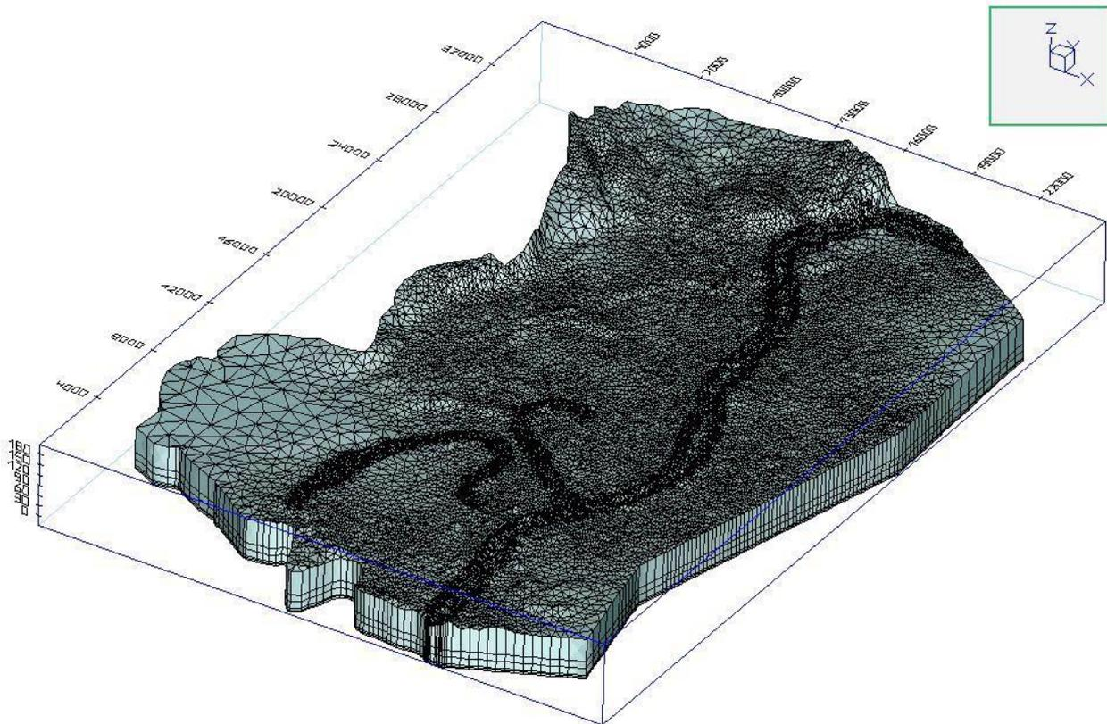
Figure 14.3.3-1: Allocation of grid points for the hydrodynamic model
