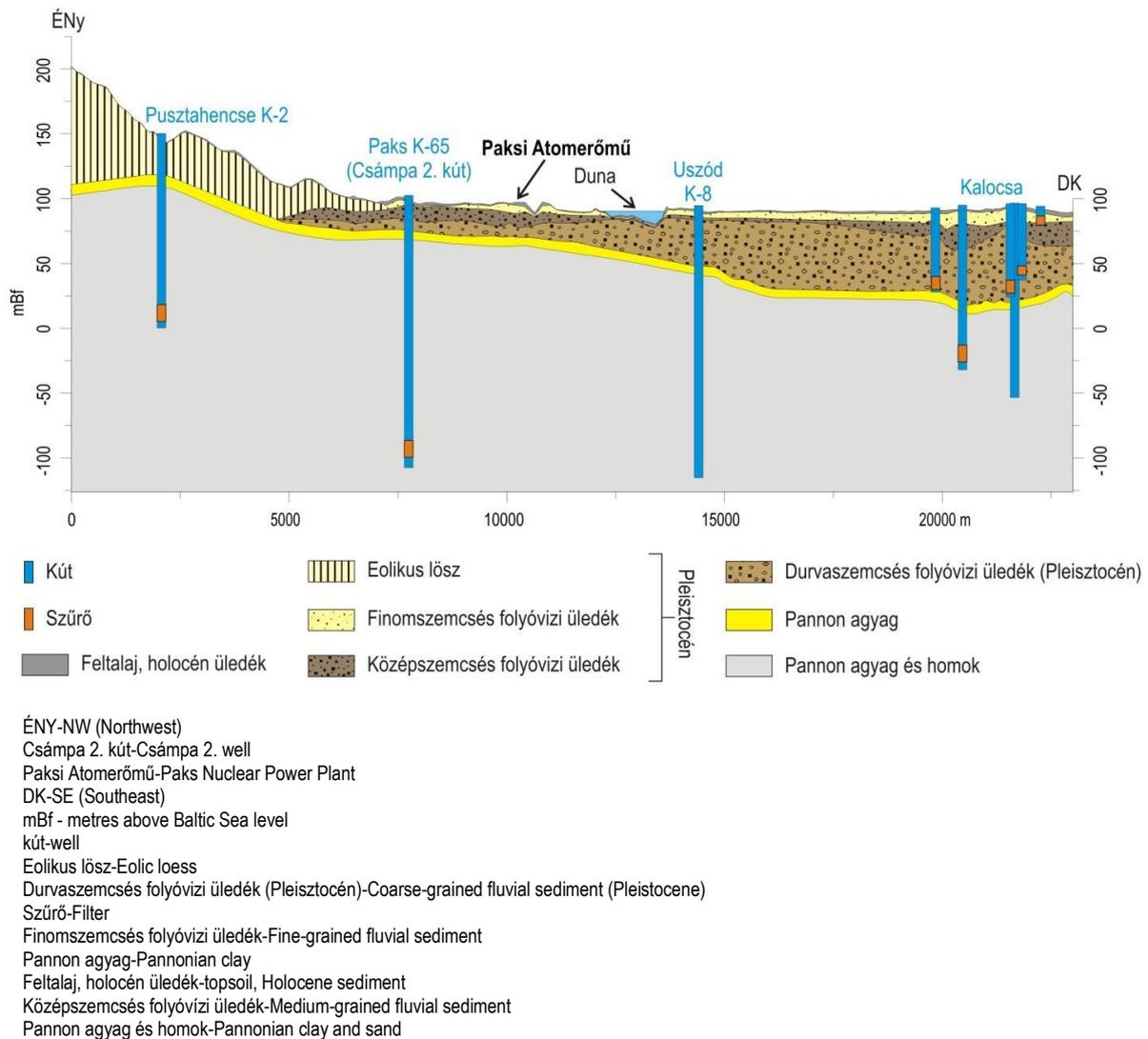
Figure 14.2.2-1: The NW-SE hydrogeological section crossing the area under study
