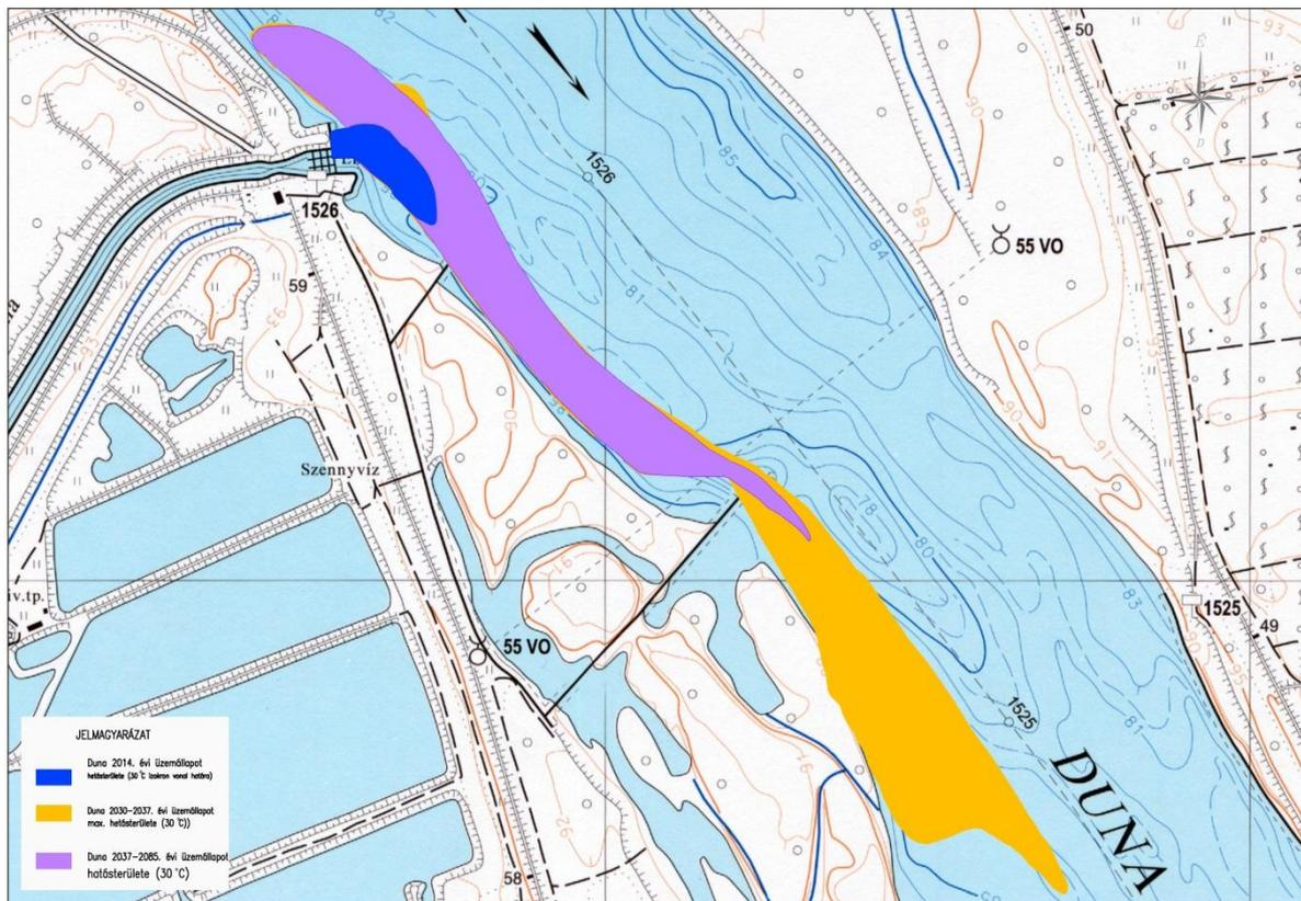
Blue area: the area of Danube water with minimum temperature of 30 °C associated with the current operating state of the Paks Nuclear Power Plant
