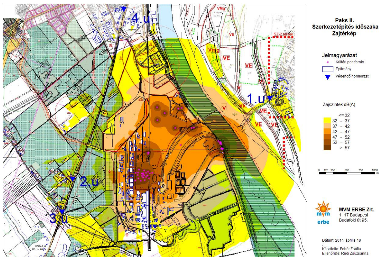
Figure 15.4.2-4: Noise load during structure construction works [15-9]
